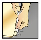
If it is necessary to remove or dismantle parquet planks, a complete row of planks must be clicked out upwards. The parquet planks can then be pushed apart flat against each other.
