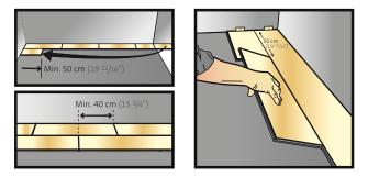
Boen parquet with click connection do not require glue indication on the profiles. In certain cases, e.g. in the event of a required the element can simply be pushed in by removing the tongue on the groove cheek. In this case, glue must be applied in this area using suitable parquet glue.
