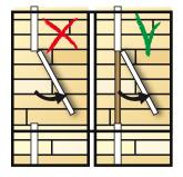
Parquet in narrow, long rooms, for example, hallways should not be laid in the transverse direction, but always in the longitudinal direction.
