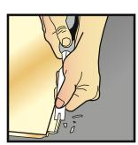
If it is necessary to remove or dismantle parquet planks, a complete row of planks must be clicked out upwards. The parquet planks can then be pushed apart flat against each other.
